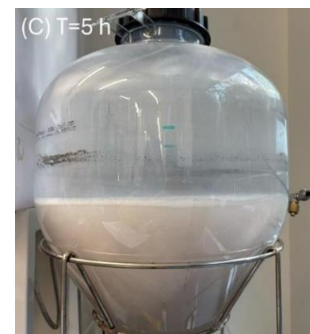
Photo 3: Foam formation at T = 5 h, after 5 hours of ozonation, a clear visual sign of active PFOS removal and foam development
